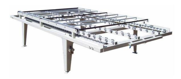
The Evans Midwest Model 0366 Index Table aligns laminate and core stock accurately. The fully adjustable design accepts materials up to 62" wide by 145" long, and is the ideal complement to the 0206 Pinch Roller. Adjustable table guides assure quick and correct spacing between core stock and backslash for the cove bend. An air supply of only 80 PSI is required.
