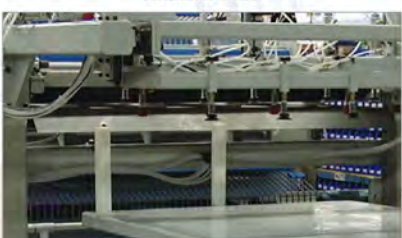
Automatic vacuum feeder for the HPL eliminating need for operator
