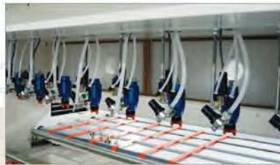
Unique spray gun design reduces overspray and misting
