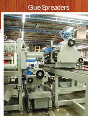
Upper and lower glue spreaders move out of operating position for ease of cleaning and maintenance
