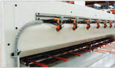
Electric sensors for automatically controlling spray width
