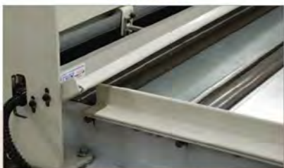
Special HPL cleaner with ionization unit, brush and vacuum pump
