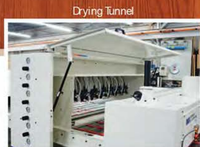
Gas spring operated access door for ease of cleaning and maintenance
