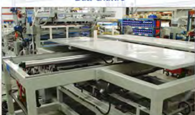
Optional dual shuttles reduce downtime and increase productivity
