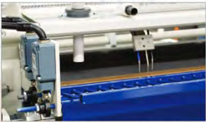
Optional automatic level sensing control to insure continuous adhesive supply to spreaders
